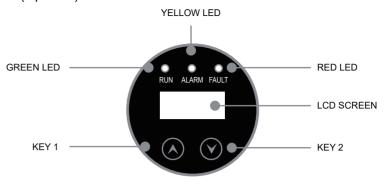
The LCD screen display module includes a display screen and two touch buttons on the front panel of the inverter, which shows the following information:
