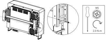
Fig 2.3 Wall mounted bracket
