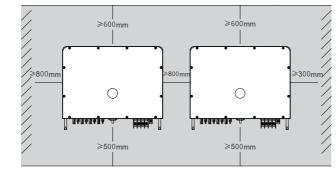
Fig. 2.0 Installation clearance of inverter
