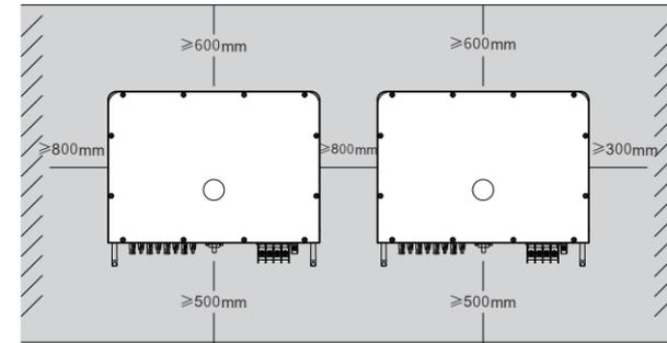
Fig. 2.0 Installation clearance of inverter
