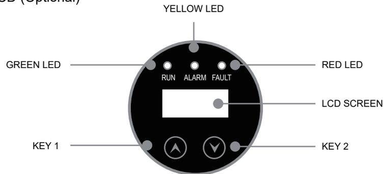
The LCD module includes a display screen and two touch keys. The function of keys are as follows:
