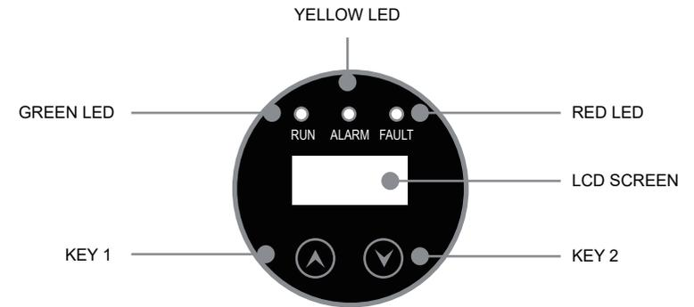
The LCD screen display module includes a display screen and two touch buttons on the front panel of the inverter, which shows the following information:
